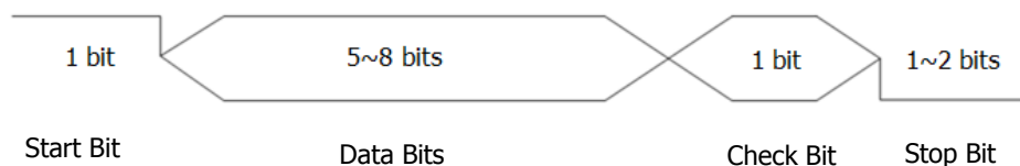
Figure 5-13 Schematic Diagram of RS232 Protocol
