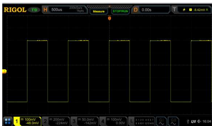
Figure 4-3 Waveforms after 128 Times of Averaging
