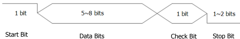
Figure 5-13 Schematic Diagram of RS232 Protocol
