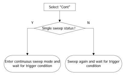
Figure 2-9 Process of Continuous Sweep
