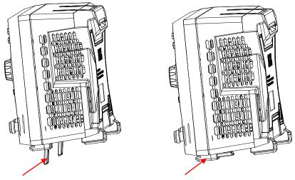
To unfold the supporting legs To fold the supporting legs Figure 1-3 To Adjust the Supporting Legs
