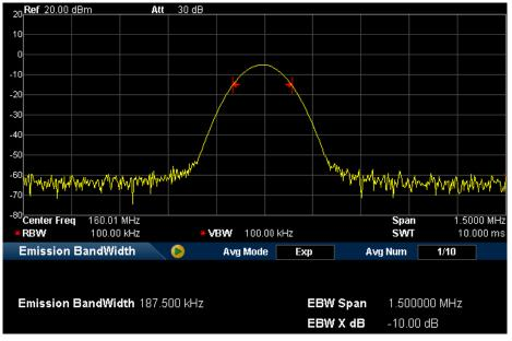
Figure 2-18 EBW Measurement Interface
