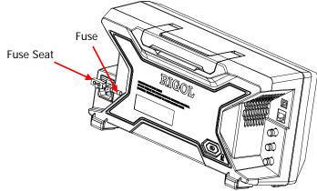
Figure 1-16 To Replace the Fuse
