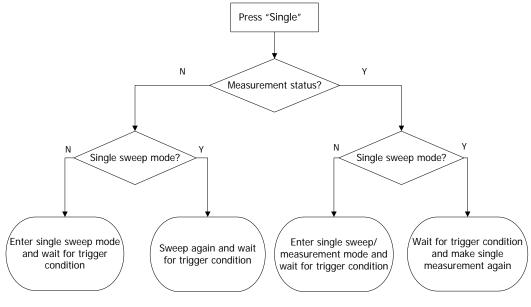
Figure 2-10 Process of Single Sweep
