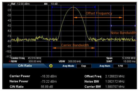
Figure 2-19 C/N Ratio Measurement Interface
