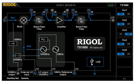
Figure 2-31 TX1000 control panel
