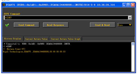
Figure 3-2 Write and Read Commands via USB
