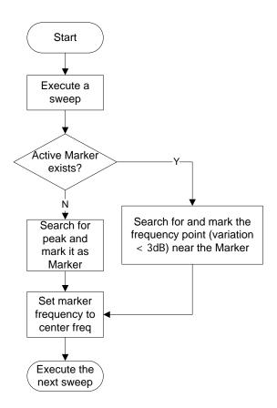
Figure 2-1 Process of Signal Track
