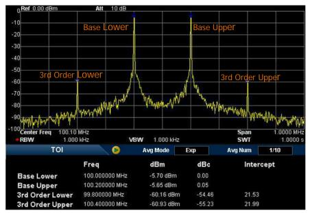
Figure 2-21 TOI Measurement Interface
