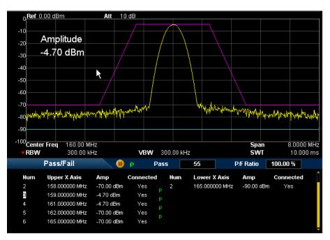
Figure 2-11 Interface of Pass/Fail Test
