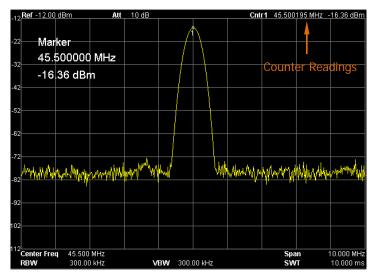
Figure 2-26 Frequency Counter Measurement
