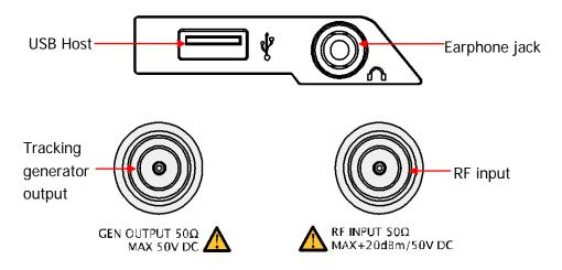
Figure 1-7 Front Panel Connectors
