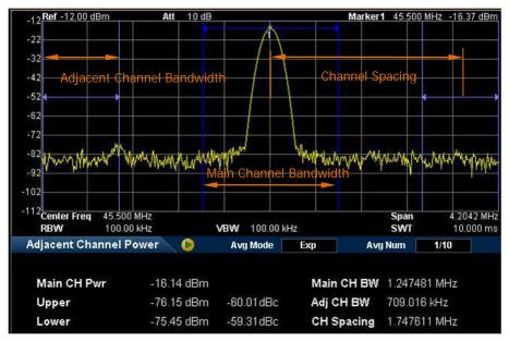
Figure 2-15 Adjacent Channel Power Measurement Interface
