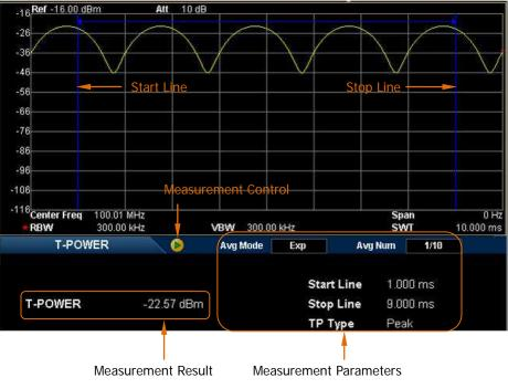
Figure 2-14 T-Power Measurement Interface
