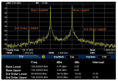
Figure 2-19 TOI Measurement Interface
