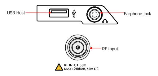
Figure 1-7 Front Panel Connectors
