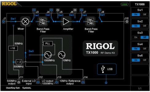
Figure 2-29 TX1000 control panel
