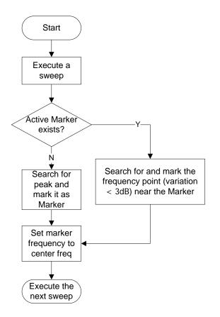
Figure 2-1 Process of Signal Track
