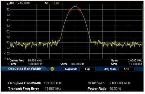
Figure 2-15 OBW Measurement Interface
