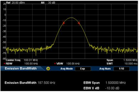
Figure 2-16 EBW Measurement Interface
