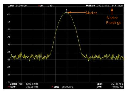
Figure 2-21 Schematic of the Marker
