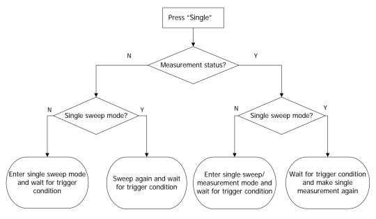
Figure 2-10 Process of Single Sweep
