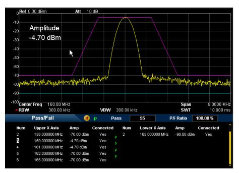
Figure 2-11 Interface of Pass/Fail Test
