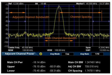
Figure 2-13 Adjacent Channel Power Measurement Interface
