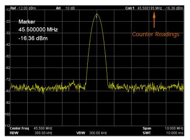
Figure 2-24 Frequency Counter Measurement
