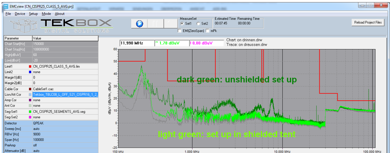
Picture 6: CISPR 25 conducted noise measurement; DUT powered
