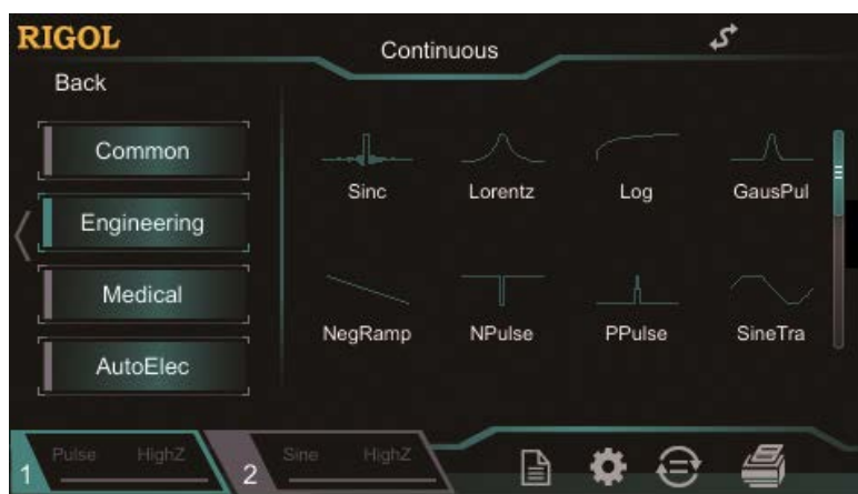
Figure 2-4 Arbitrary Waveform Selection Interface
