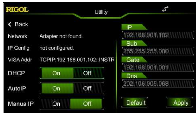
Figure 2-26 LAN Setting Interface
