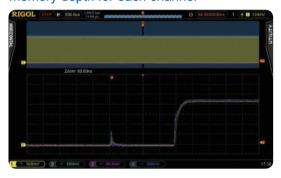
Provide the capability to see both the panorama and detail simultaneously.
